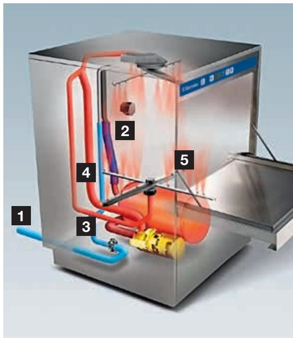
The **air-break** prevents water from flowing back into the mains in case of machine failure and stabilizes water pressure.
